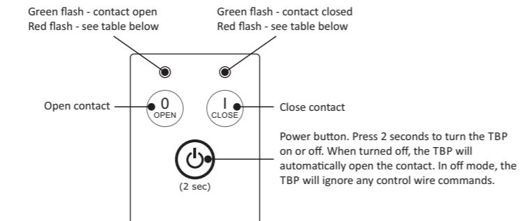
During normal operation a green flashing LED indicates whether the TBP contact is open or closed. This contact state can be changed by pressing the local OPEN and CLOSE buttons, or through the remote control wires.
